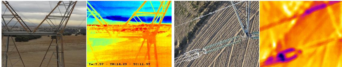
**Figure 13.** High voltage tower pictures, from left to right: optical-lateral, thermal-lateral, optical-zenit and thermal-zenit.
