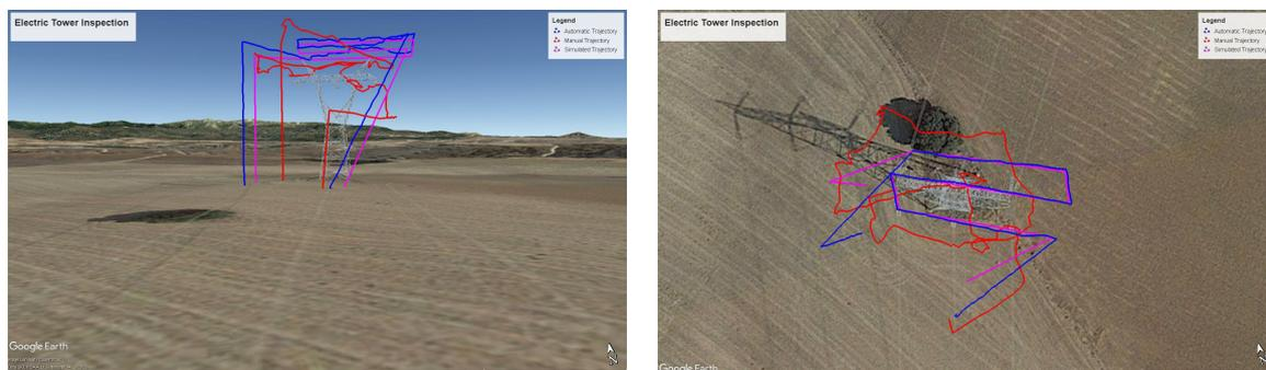
**Figure 10.** Manual (red), automated (blue) and MDS simulated/predicted (magenta) 3D trajectory: (left) lateral, (right) zenit.
