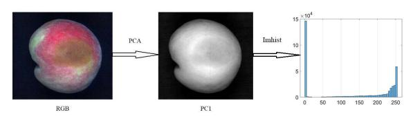
Figure 4. The common procedure for image processing.
