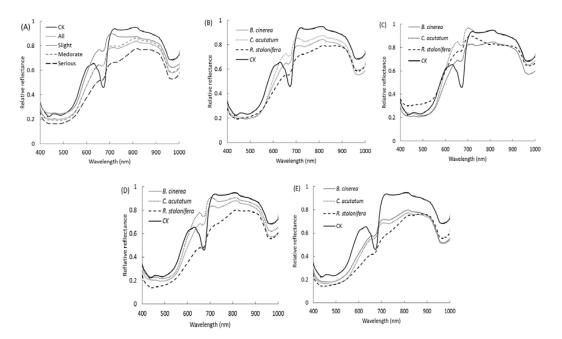
**Figure 2.** Average reflectance spectra of three kinds of disease and control group using the entire spectral region from 400 to 1000 nm for (**A**) different decay stages of all kinds of diseases, (**B**) different kinds of diseases of all decay stages, (**C**) slightly-decayed samples of different diseases, (**D**) moderately-decayed samples, (**E**) severely-decayed samples.
