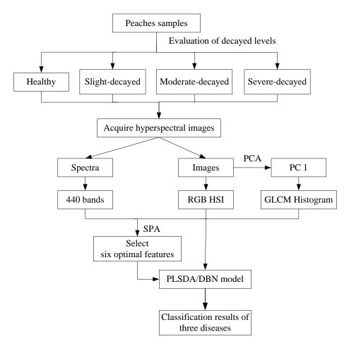
**Figure 1.** Flowchart of the data analysis procedures used to classify different fungal diseases. (PCA: principal components analysis; PC1: first principal component image; SPA: successive projections algorithm; RGB: red, blue, and green; HIS: hue, saturation, and lightness; GLCM: gray level co-occurrence matrix; PLSDA: partial least squares discrimination analysis; DBN: deep belief network).
