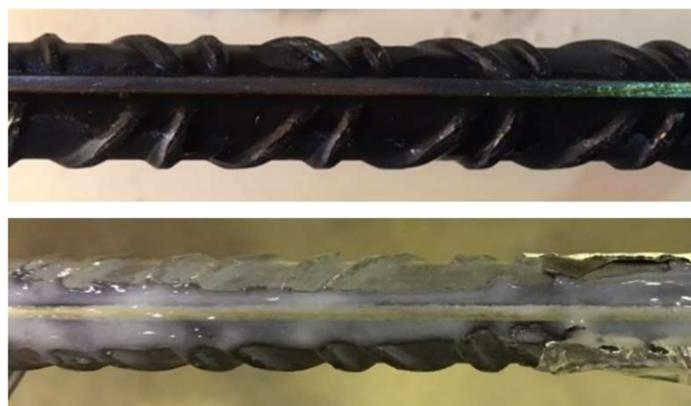
**Figure 9.** Adhesives on rebar of each beam specimen: cyanoacrylate (Beam 1—top), two-component epoxy (Beam 2—bottom).
