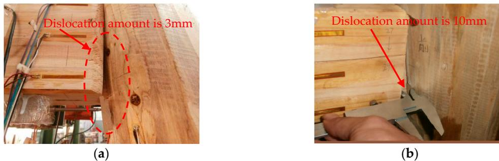
**Figure 16.** Measured dislocation with a: (a) loading amplitude of 80 mm; (b) loading amplitude of 160 mm.
