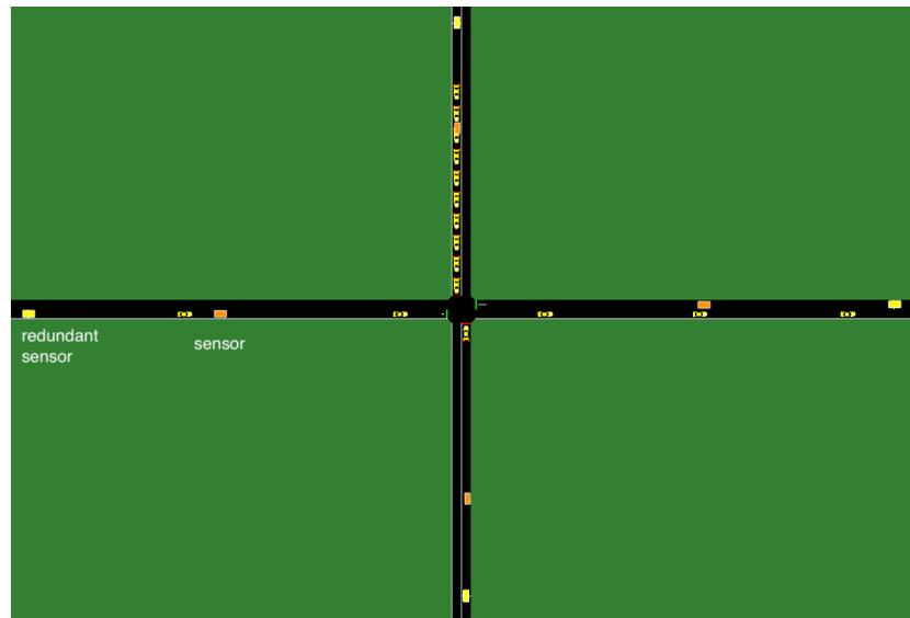
**Figure 5.** Each intersection in the 3-by-3 grid. For illustration, a critical and a redundant sensor are shown in the figure. For each lane, a second redundant sensor is placed with twice as much distance as the distance between the first redundant sensor and the critical sensor. All 8 total redundant sensors are used to predict the value of a sensor.
