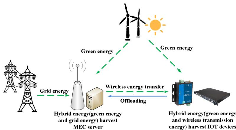
**Figure 2.** A multi-user multi-task MEC system with hybrid energy harvesting.
