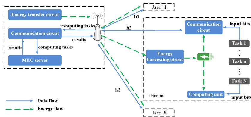
**Figure 1.** The detailed multi-user multi-task MEC (Mobile Edge Computing) system architecture when only considering IoT (Internet of Things) devices with wireless powered model.
