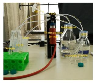
Figure 14. Configuration of the thermostated syringe.
