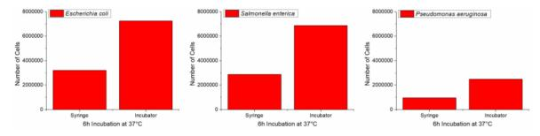
**Figure 15.** Results of the incubations in the thermostated syringe compared to respective bacteria incubations in the bacteriological incubator.
