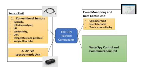
Figure 7. Configuration of WaterSpy based on TRITON platform.
