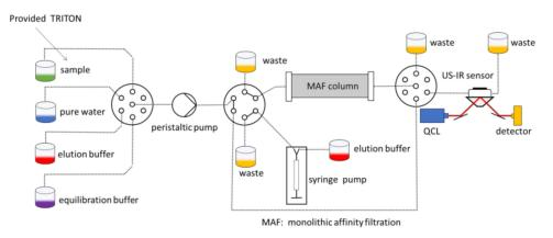
Figure 9. Details of the sample handling and pre-concentration system.
