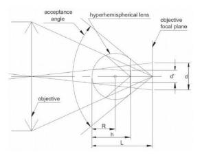
Figure 8. The GaAs hyperhemispherical lens.
