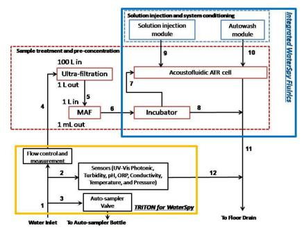
Figure 6. Integrated WaterSpy fluidic system.
