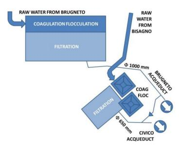
Figure 3. Schematic diagram of the water flow.
