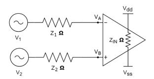
Figure 3. Skin, electrode, and amplifier interface electrical model.
