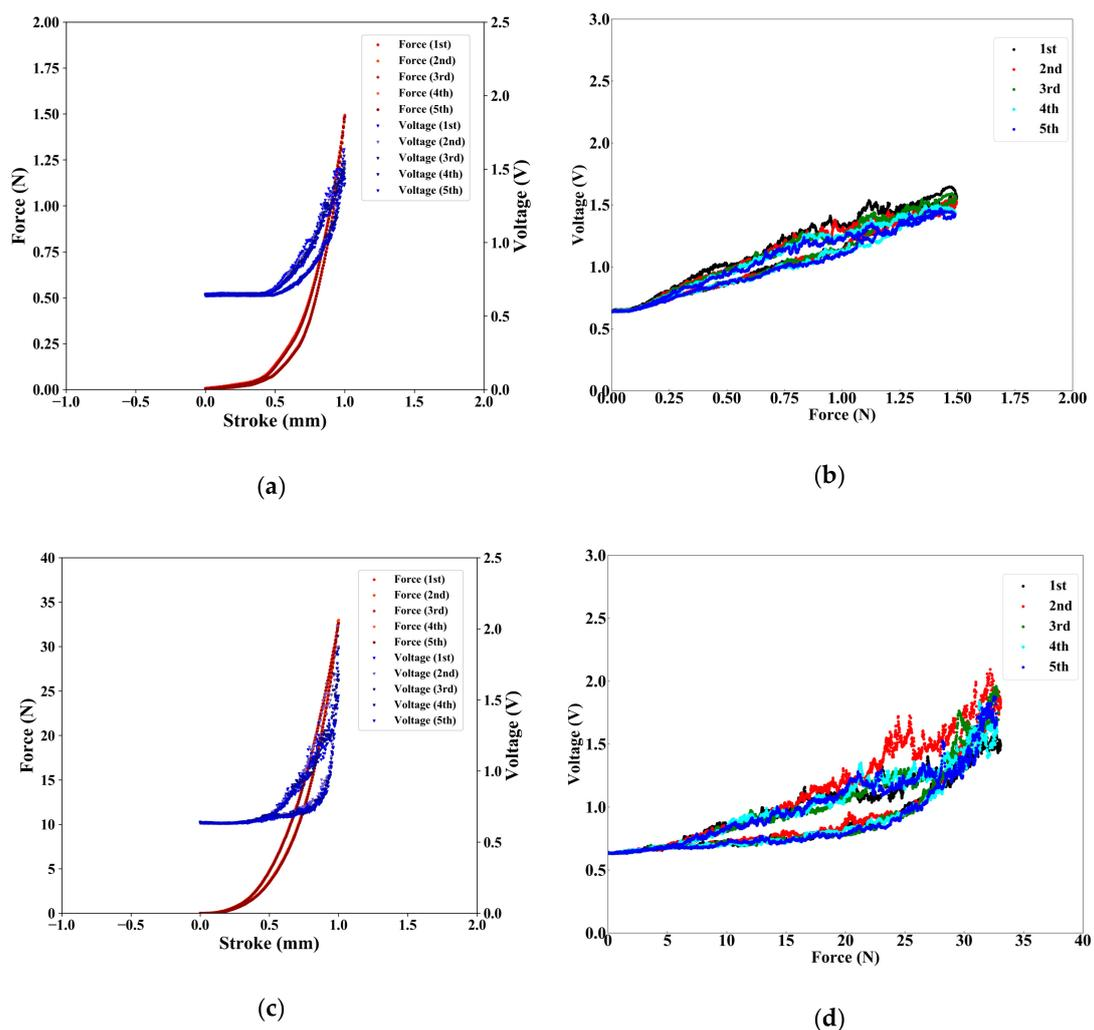
**Figure 5.** Results of evaluation of hysteresis. (a) Changes of force (from a reference value) and voltage in soft-MPS (soft) vs. stroke (1 mm/s). (b) Change of voltage in soft-MPS (soft) vs. force. (c) Changes of force and voltage in soft-MPS (hard) vs. stroke (1 mm/s). (d) Change of voltage in soft-MPS (hard) vs. force.
