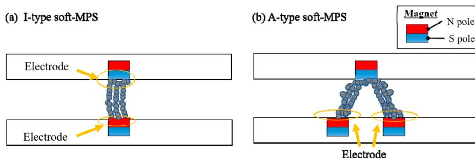
**Figure 1.** Magnetic field orientation of the ferromagnetic powder for two different types of magnetic resistive tactile sensors: (a) I-type soft-magnetic powdery sensors (MPS). One of the electrodes is set on the plate to which the external force is applied. (b) A-type soft-MPS. All electrodes are set on the bottom side.
