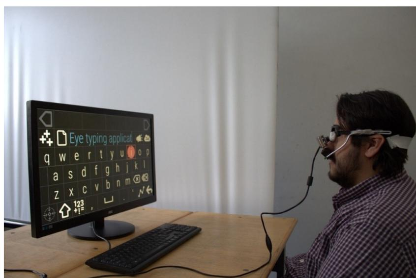
**Figure 1.** Head-mounted eye tracking interface.
