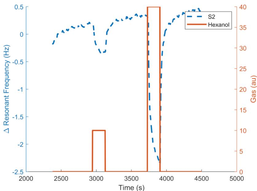
**Figure 11.** Example of frequency response of the [MOIM] [PF<sub>6</sub>] sensor for two hexanol concentrations.
