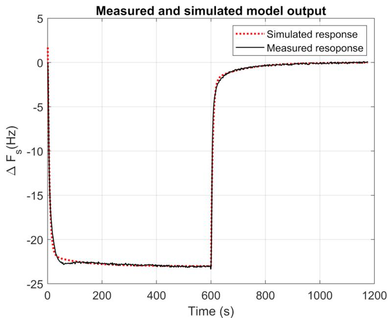
**Figure 6.** Response of a sensor at one step of hexanol (black) and its model, fitted as Equation (4) (dashed line) for the response of the [BMIM][Br] sensor to a hexanol step.
