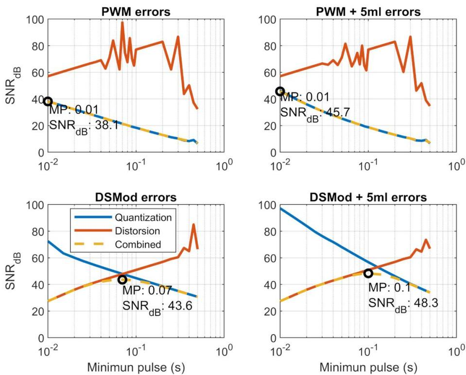
**Figure 7.** Errors of reconstruction in the different control strategies tested. The black circles represent the optimum minimum pulse (MP).
