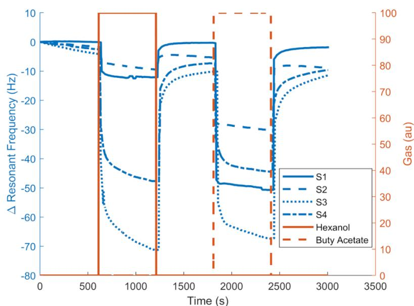
**Figure 10.** Example of frequency response of the [MOIM] [PF<sub>6</sub>] sensor for hexanol and butyl acetate.
