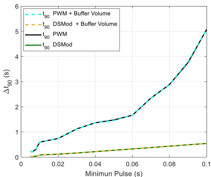
**Figure 8.** Differences of the  $t_{90}$  for the different control simulated strategies.
