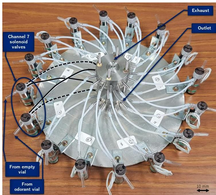
Figure 4. Detail of one assembly part of the odor generation system.
