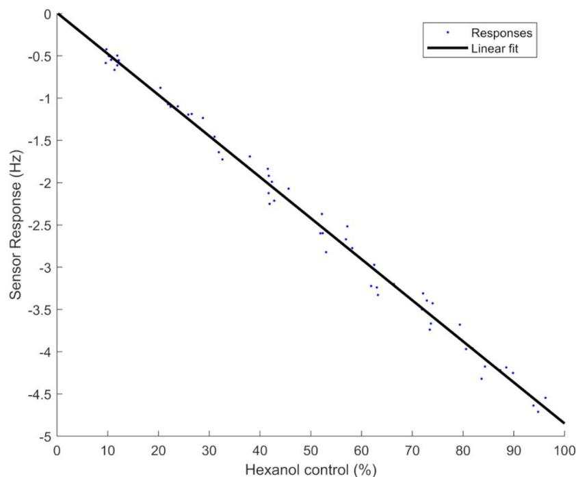
**Figure 12.** Linear adjustment of all compensated concentration percentages produced by all channels.
