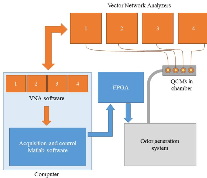
**Figure 1.** Scheme of the artificial olfactory system.
