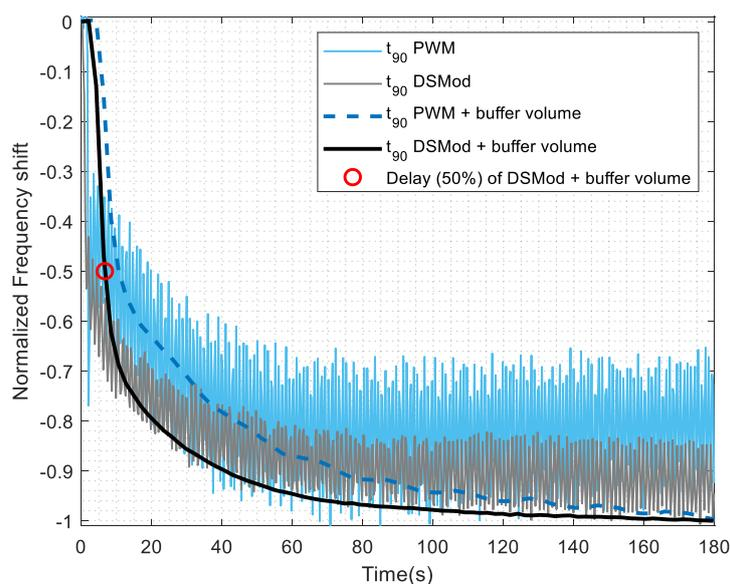
**Figure 9.** Effect of the different control strategies for the [BMIM][Br] sensor to hexanol at 50% controlled concentration percentage. Conditions of the measurements were made at a minimum pulse of 0.01 s for PWM and a minimum pulse of 0.1 s for the delta-sigma modulator, and a buffer volume of 5 mL was used.
