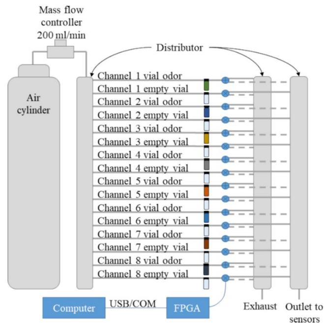
Figure 3. Scheme of the odor generation system.
