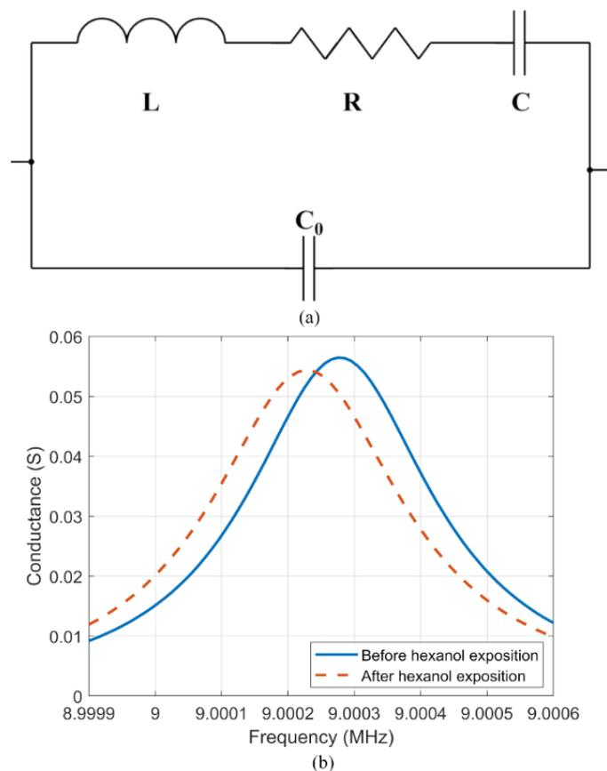
**Figure 2.** Behavior of the QCM. (a) Mason equivalent circuit. (b) Measured frequency characteristic for the QCM sensor coated with [BMIM][Cl] before (solid line) and after (dashed line) exposure to hexanol.
