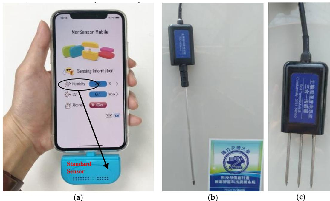
**Figure 15.** Smartphone-based portable STD value generator; (a) STD sensors in the air; (b) and (c) STD sensors in the soil.
