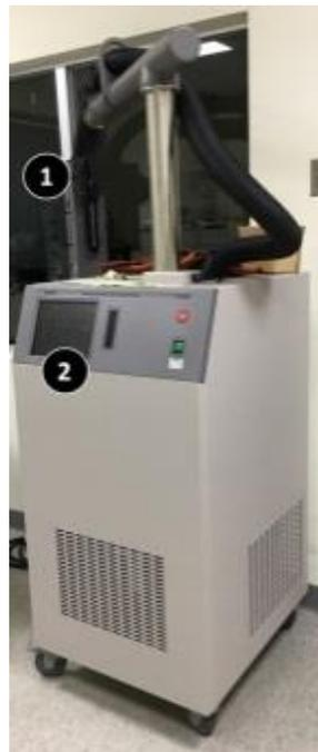
Figure 3. The Thermonics T-2500SE temperature forcing system.
