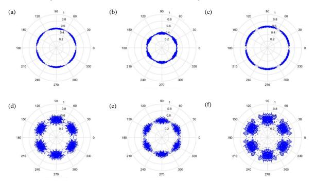
**Figure 9.** Results by improved formula when t = 1 and sampling is at 1000 Hz/1000 rpm. (a) Normal, (b) motor platform with one eccentric screw, (c) motor platform with two eccentric screws, (d) sanded ball bearings, (e) insufficient lubrication, and (f) worn ball bearings.
