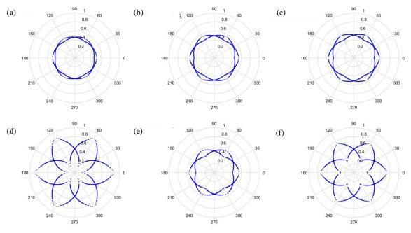
**Figure 16.** Results from improved formula when t = 0 and sampling is at 3000 Hz/2000 rpm. (a) Normal, (b) motor platform with one eccentric screw, (c) motor platform with two eccentric screws, (d) sanded ball bearings, (e) insufficient lubrication, and (f) worn ball bearings.
