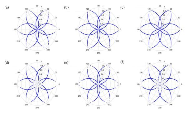
**Figure 14.** Results from improved formula when t = 0 and sampling is at 3000 Hz/2000 rpm. (a) Normal, (b) motor platform with one eccentric screw, (c) motor platform with two eccentric screws, (d) sanded ball bearings, (e) insufficient lubrication, and (f) worn ball bearings.
