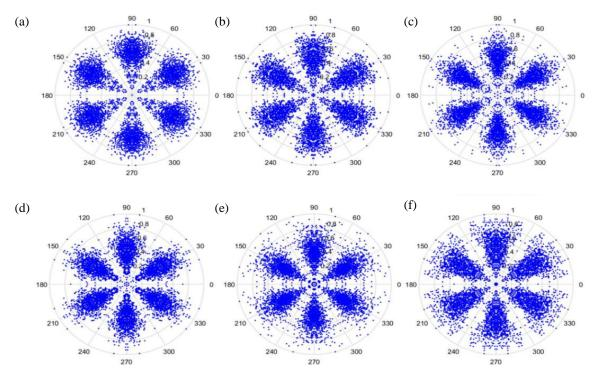
**Figure 7.** Results when t = 1 and sampling is at 1000 Hz/1000 rpm. (a) Normal, (b) motor platform with one eccentric screw, (c) motor platform with two eccentric screws, (d) sanded ball bearings, (e) insufficient lubrication, and (f) worn ball bearings.
