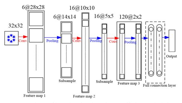
Figure 13. Architecture of the convolutional neural network (CNN) used for the proposed method.
