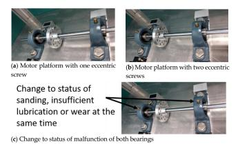
Figure 3. Malfunction simulation schematic.
