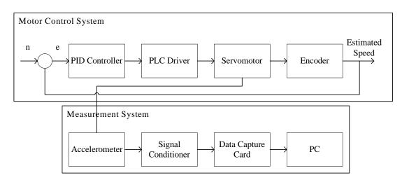
Figure 1. System structure.
