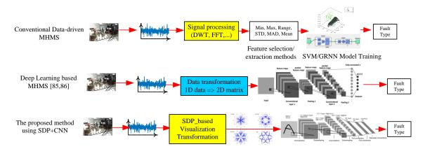
**Figure 10.** Comparison between the conventional data-driven machine-health monitoring systems (MHMS), the deep-learning-based MHMS, and the proposed method.
