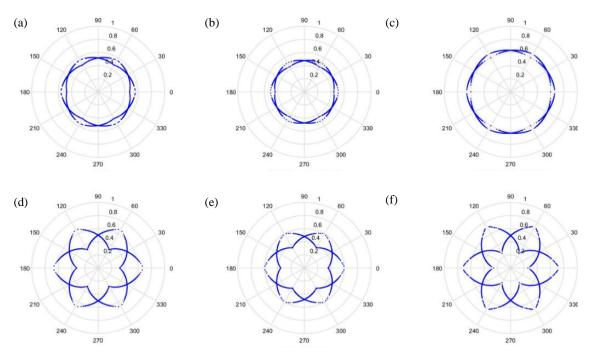
**Figure 8.** Results by improved formula when t = 0 and sampling is at 1000 Hz/1000 rpm. (a) Normal, (b) motor platform with one eccentric screw, (c) motor platform with two eccentric screws, (d) sanded ball bearings, (e) insufficient lubrication, and (f) worn ball bearings.
