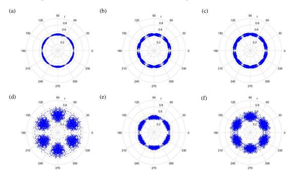
**Figure 17.** Results from improved formula when t = 1 and sampling is at 3000 Hz/2000 rpm. (a) Normal, (b) motor platform with one eccentric screw, (c) motor platform with two eccentric screws, (d) sanded ball bearings, (e) insufficient lubrication, and (f) worn ball bearings.
