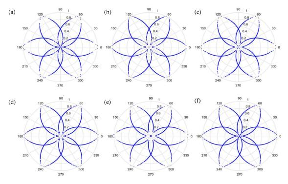
**Figure 6.** Results when t = 0 and sampling is at 1000 Hz/1000 rpm. (a) Normal, (b) motor platform with one eccentric screw, (c) motor platform with two eccentric screws, (d) sanded ball bearings, (e) insufficient lubrication, and (f) worn ball bearings.
