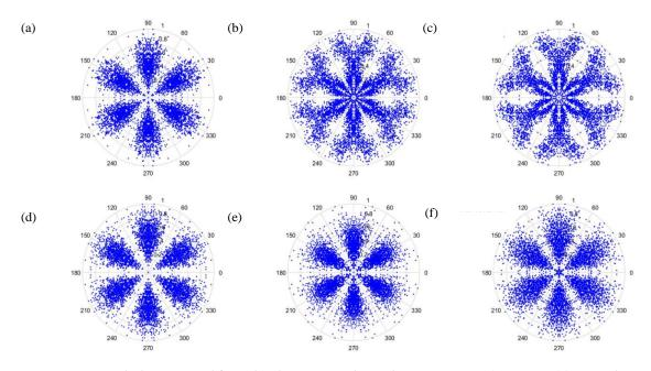
**Figure 15.** Results by improved formula when t = 1 and sampling is at 3000 Hz/2000 rpm. (a) Normal, (b) motor platform with one eccentric screw, (c) motor platform with two eccentric screws, (d) sanded ball bearings, (e) insufficient lubrication, and (f) worn ball bearings.
