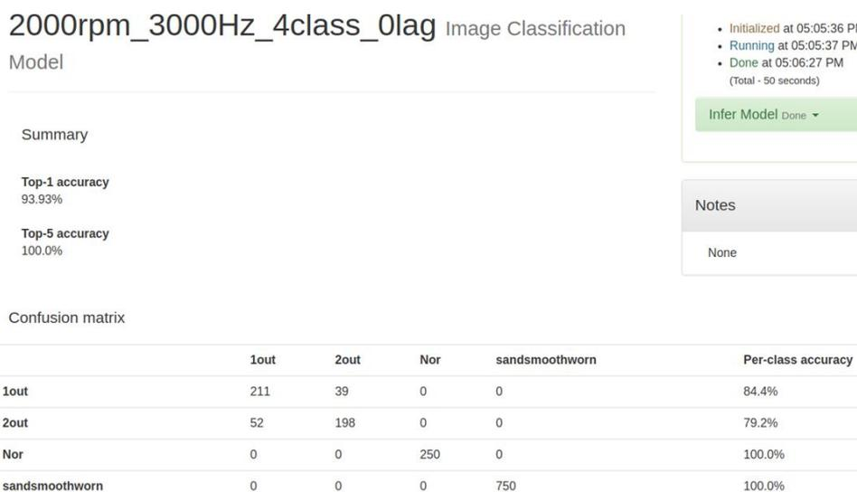
**Figure 18.** Confusion matrix for the improved formula of symmetrized dot pattern (SDP) as (sampling at 3000 Hz/2000 rpm).
