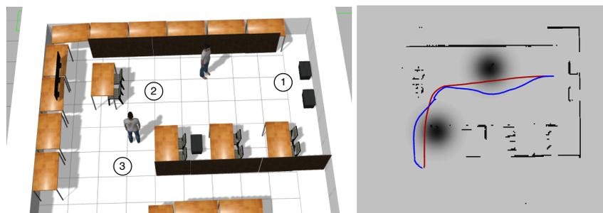
**Figure 9.** (Left) Experiment 1 setup with the reference waypoints. The robot started at Waypoint 1, went to Waypoint 2 and finished at Waypoint 3. (Right) Path for ROS traditional navigation in red and the path followed with our approach in blue.
