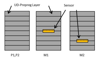
Figure 3. Schematic of the different samples uses. The dimensions are not in scale. The thickness of the prepreg layers is around 2 mm while the sensor thickness is approximately 6  $\mu$ m. The fibers are oriented unidirectionally. The fibers direction is along the out of plane axis.
