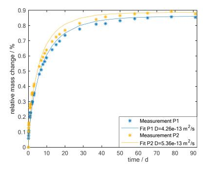
**Figure 4.** Mass change of two CFRP samples (see Table 2) with resin M21 during exposure to a hot-wet environment of 70°C and 85% relative humidity.
