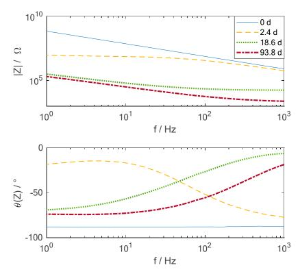
**Figure 5.** Amplitude and phase over frequency of the impedance of the interdigital sensors S2 integrated into the CFRP during exposure to a hot-wet environment of 70°C and 85% relative humidity for different times.
