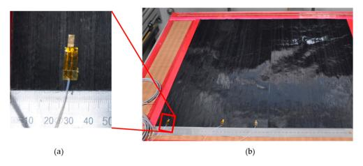
**Figure 2.** (a) Sensor during the integration in carbon fiber composite. (b)Carbon fiber prepreg plate with sensors during fabrication.
