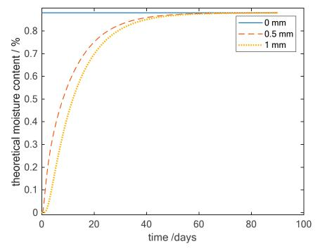
Figure 7. Theoretical mass change at the positions of the sensors S1 (1 mm) and S2 (0.5 mm).
