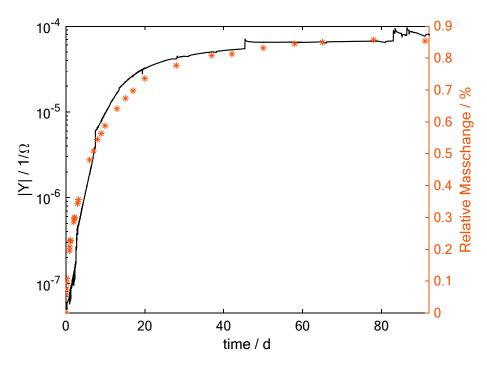
**Figure 8.** Amplitude of admittance changes Sensor S2 compared to the mass change during hot-wet test. Here the measurement at a frequency of 31.6 Hz is shown.
