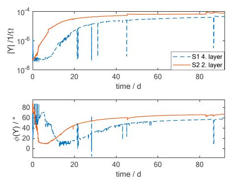
**Figure 6.** Admittance changes of two interdigital sensors integrated into the CFRP at a different position during exposure to a hot-wet environment of 70 °C and 85 % relative humidity. Here the measurement at a frequency of 31.6 Hz is shown. Sensor S1 is placed in the middle of the plate and S2 at  $\frac{1}{4}$  of the plate.
