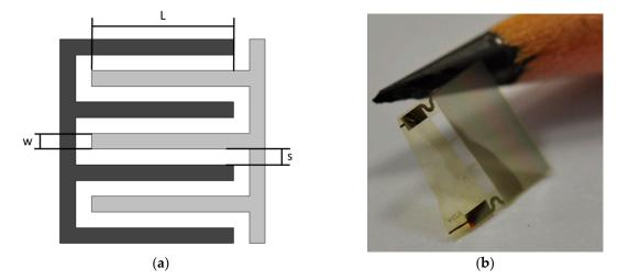
**Figure 1.** (a) Schematic of the interdigital sensor. (b) Photograph of the sensor compared to a pencil tip. The sensor area is  $3 \text{ mm} \times 6 \text{ mm}$ .
