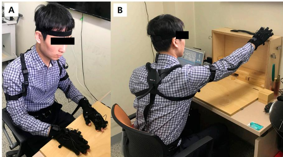
**Figure 1.** (A) A volunteer subject is wearing the IMU-based upper extremity motion capture system. (B) The subject is performing a task in the Action Research Arm Test.
