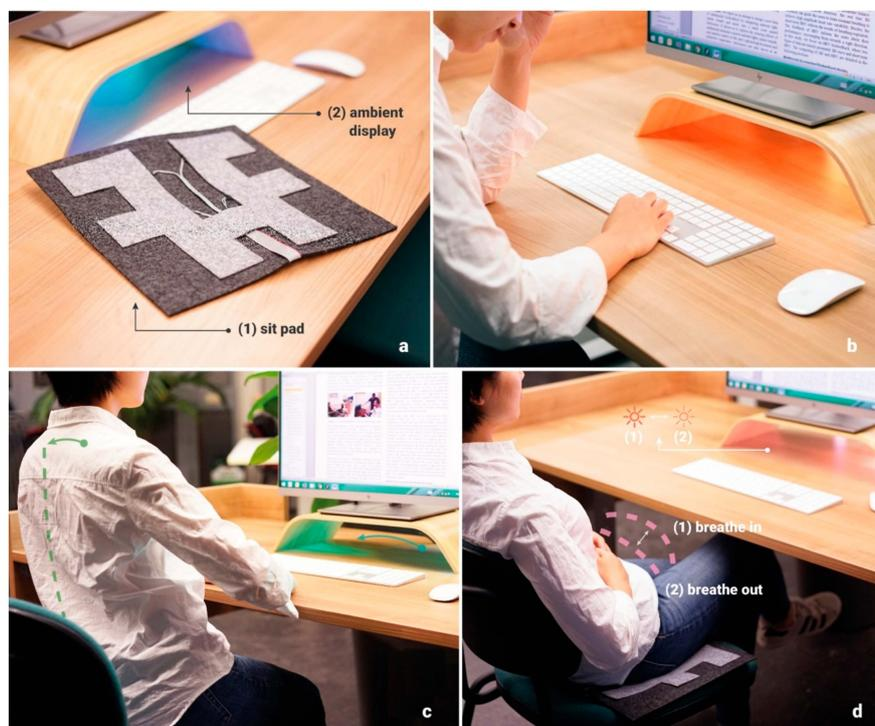
**Figure 1.** (a) LightSit comprises two parts: (1) A sit pad with pressure sensors and (2) an ambient lighting display. (b) The peripheral intervention of LightSit: When the user is overstressed and sitting for an extended period, the light becomes brighter and more saturated. (c) Stretching fitness: The light waves between left and right to mirror movement. (d) Deep breathing relaxation: The light (1) rises and (2) falls to mimic breathing patterns.
