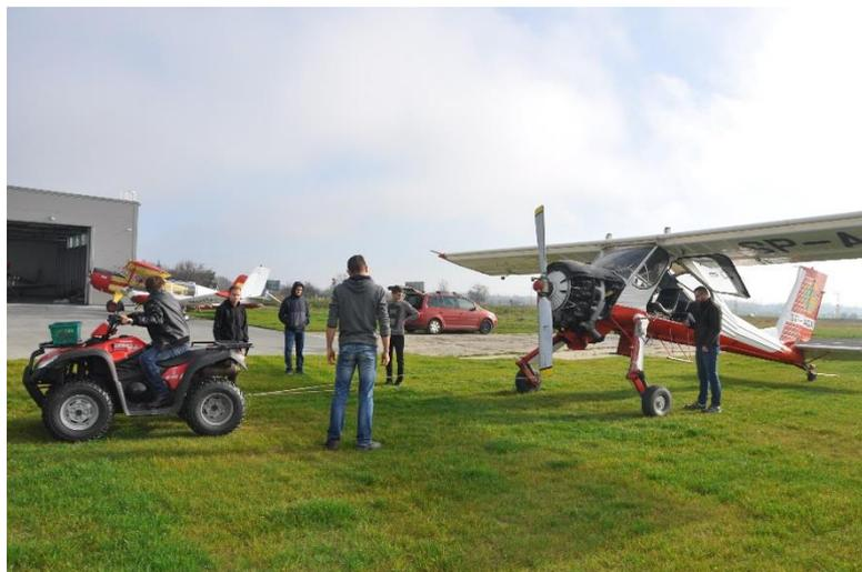
**Figure 8.** Starting a test run. The test airplane is pulled by an all-terrain vehicle (ATV). The test engineer is walking by the test airplane, collecting data wirelessly. Four persons onboard the airplane.
