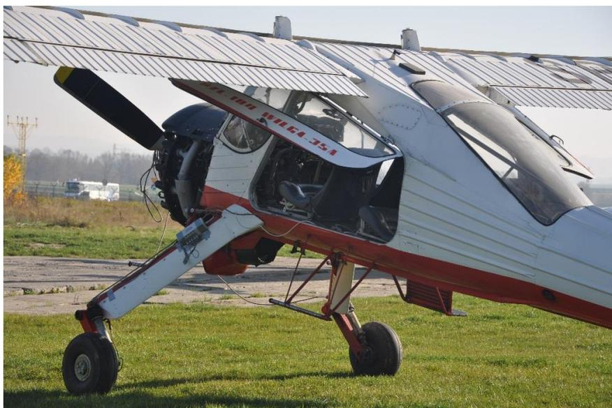
**Figure 5.** The wheel force sensor installed on the test airplane, ready for the tests.
