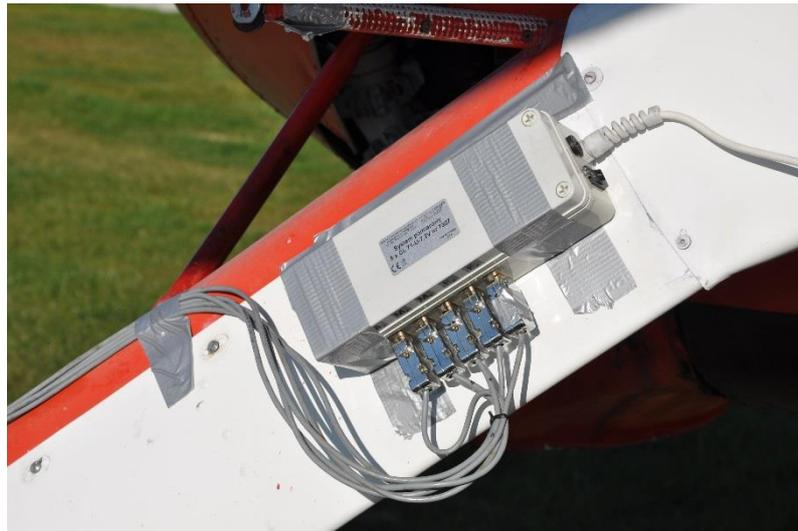
**Figure 6.** The electronics: Signal amplifiers and wireless data transfer system in the box, installed on the landing gear leg (a silver tape was used for quick installation).
