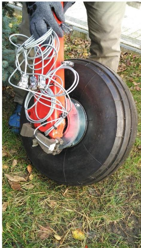
**Figure 2.** The complete wheel force sensor.
