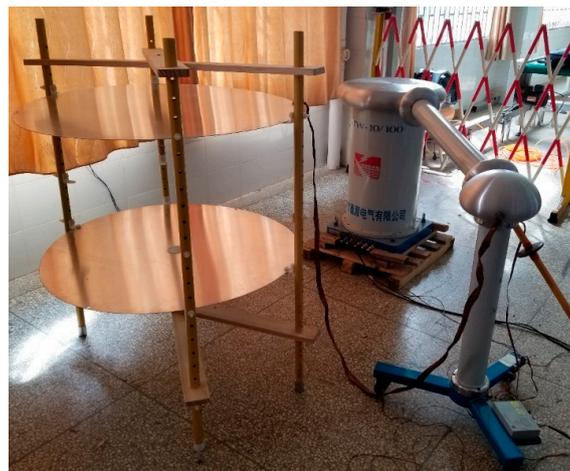
Figure 18. Power frequency voltage division ratio calibration platform.
