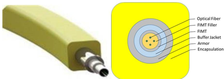
**Figure 2.** Permanent optical cable design and components [21].
