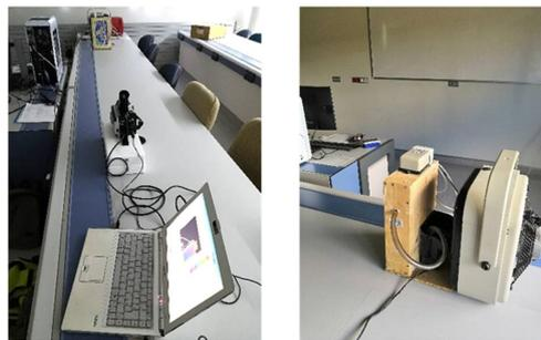
**Figure 3.** Experimental setup: relative positions of the sample, the stove and the thermographic camera, in transmission mode.
