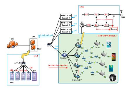
**Figure 1.** FiWi architecture illustration of the time and wavelength division multiplexed passive optical network (TWDM-PON) backhaul exploiting the power over fiber (PoF) and wireless mesh network (WMN) frontend.
