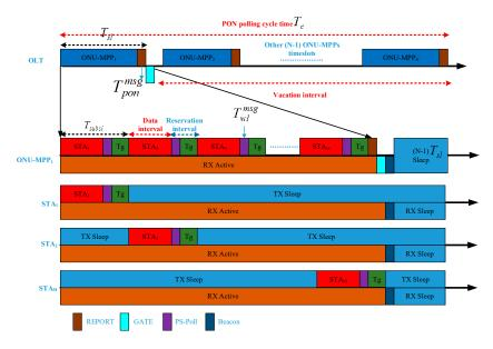
Figure 2. Power-saving illustration of the FiWi access network.
