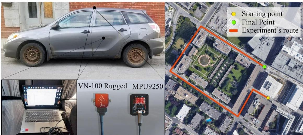
Figure 7. Dynamic experiment’s equipment and the experiment’s path.
