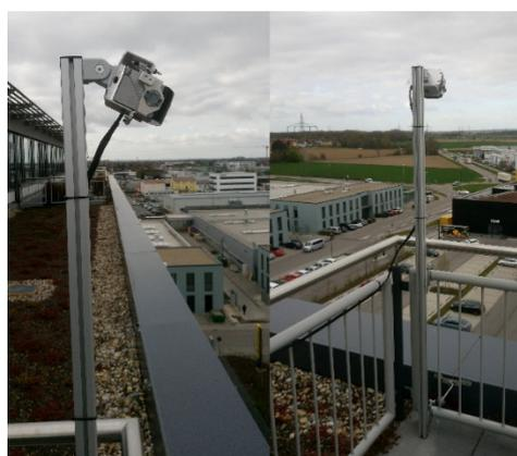
**Figure A1.** Measurement setup showing the placement of the LIDAR sensor. The location was chosen to avoid the influence of dust caused by cars and local weather variations caused by nearby high buildings or other structures.
