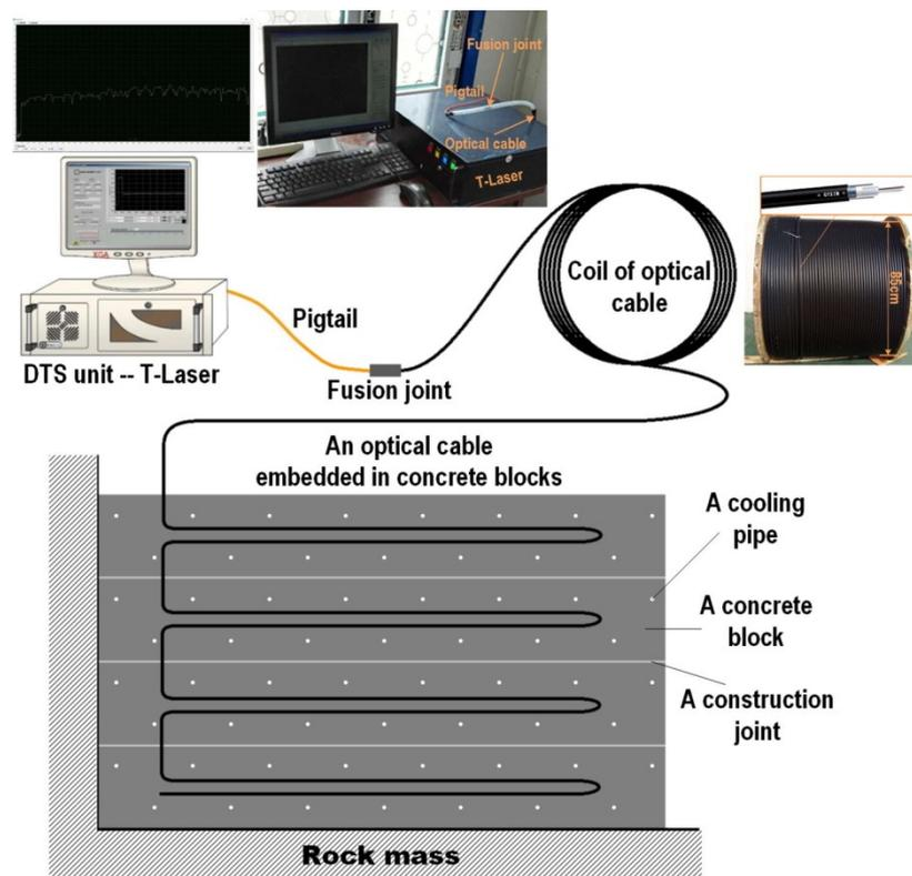
**Figure 5.** The diagram of the distributed temperature sensing (DTS) system [131].
