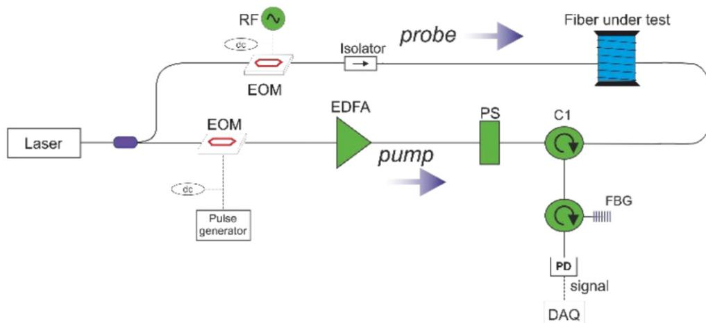
**Figure 16.** Experimental setup for distributed measurement of temperature in optical fibers. EOM: electro-optic modulator; PS: polarization scrambler; EDFA: erbium-doped fiber amplifier; PD: photodetector; FBG: fiber Bragg grating [159].
