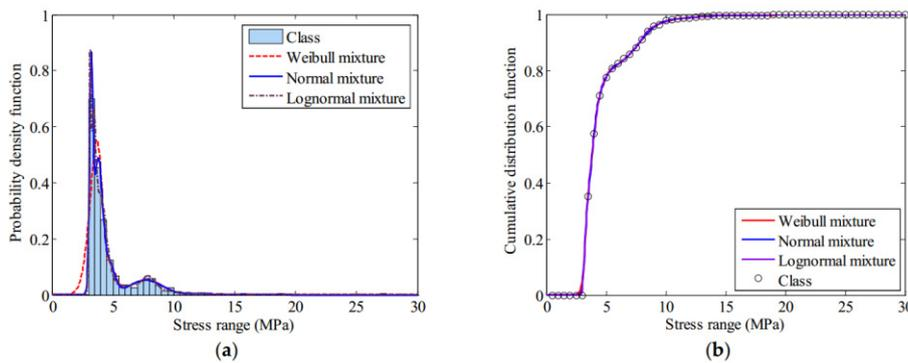
**Figure 10.** Distribution function of stress range: (a) finite mixture probability distribution function (PDF); (b) finite mixture cumulative distribution function (CDF) [151].
