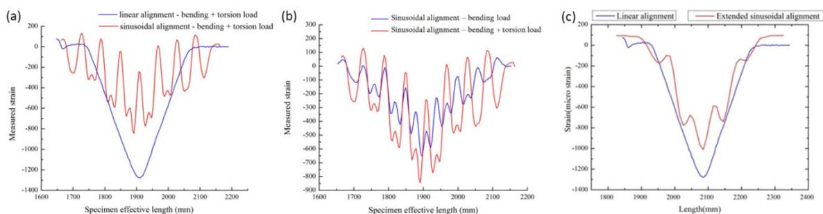
**Figure 7.** (a) Linear vs. sinusoidal alignment, bending + torsional load; (b) sinusoidal alignment, bending load with torsion vs. without torsion; (c) linear vs. extended sinusoidal alignment, bending load [139].
