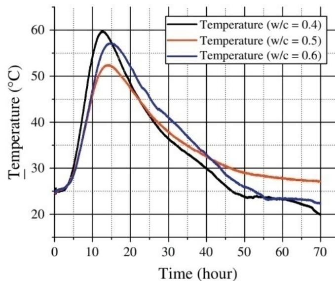
**Figure 4.** Concrete hydration experiment with water versus cement ratio 0.4, 0.5, and 0.6 using the thermocouple [65].
