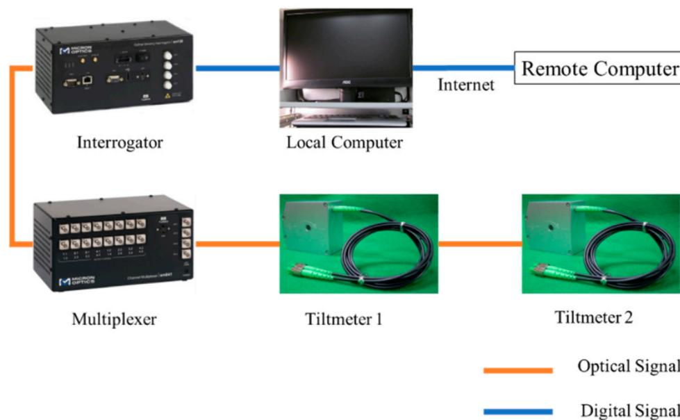
**Figure 8.** Configuration of the fiber Bragg grating (FBG) inclinometer monitoring system [147].
