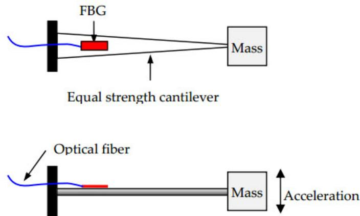
**Figure 12.** Structural schematic diagram of the designed fiber Bragg grating (FBG) sensor [152].
