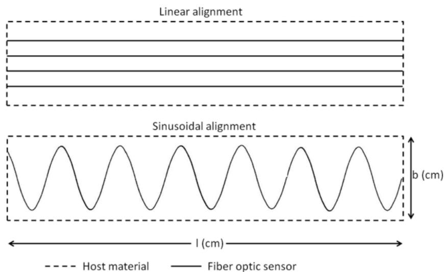
**Figure 6.** Fiber-optic sensor (FOS) installation method for a reference surface area [139].
