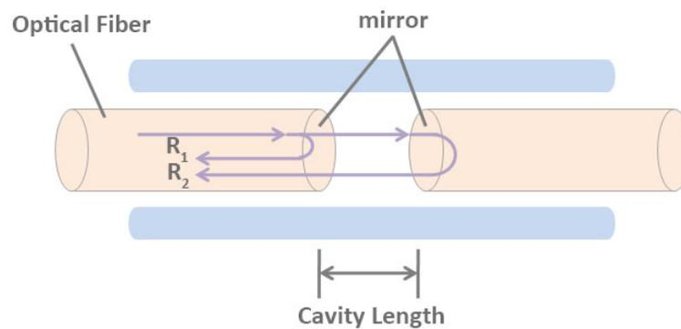
**Figure 1.** Schematic diagram of Fabry–Perot interference cavity.
