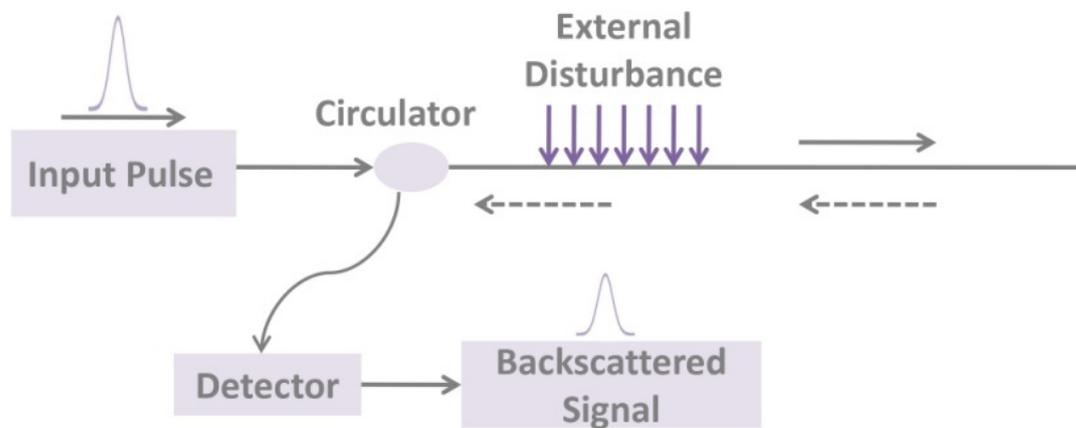
**Figure 3.** The principle of optical time-domain reflectometer (OTDR) based on backscattering.
