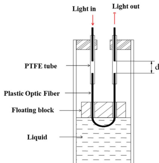
**Figure 15.** Fiber-optic-based liquid sensor setup. Note: PTFE = polytetrafluoroethylene [154].
