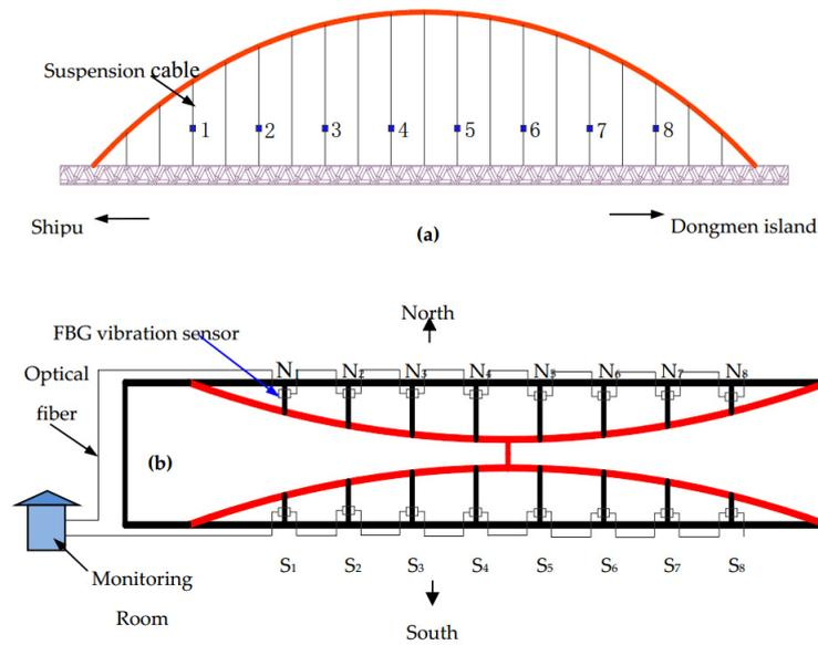
**Figure 11.** Arrangement of fiber Bragg grating (FBG) vibration sensors on Tongwamen bridge cables: (a) side view; (b) overhead view [152].
