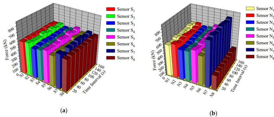
**Figure 14.** Suspension cable force distribution data measured by fiber Bragg grating (FBG) sensors: (a) south side suspension cables; (b) north side suspension cables [152].
