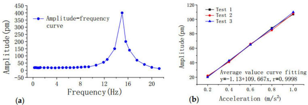
**Figure 13.** Performance test of the fiber Bragg grating (FBG) vibration sensor: (a) amplitude-frequency curve; (b) acceleration characteristics curve [152].
