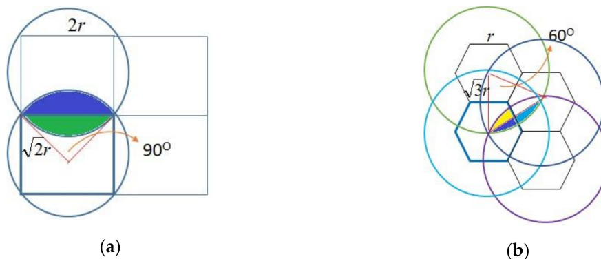
Figure 7. (a) An area monitored by two neighboring sensors in mechanisms EERH and CoDet; (b) an area monitored by four neighboring sensors in proposed mechanism, SSRM.
