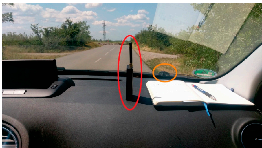
Figure 3. Position of the battery jammer (red ellipse) on the front panel and the GNSS receiver's (Ublox, NEO 6T) patch antenna on outer windscreen surface (orange ellipse) (own study).
