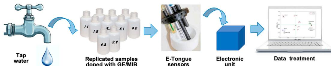
Figure 2. Schematic presentation of the employed measurement system.
