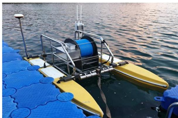
Figure 1. System structure of the unmanned surface vehicle (USV) system.
