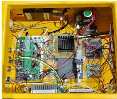
**Figure 2.** The control box of the USV system.
