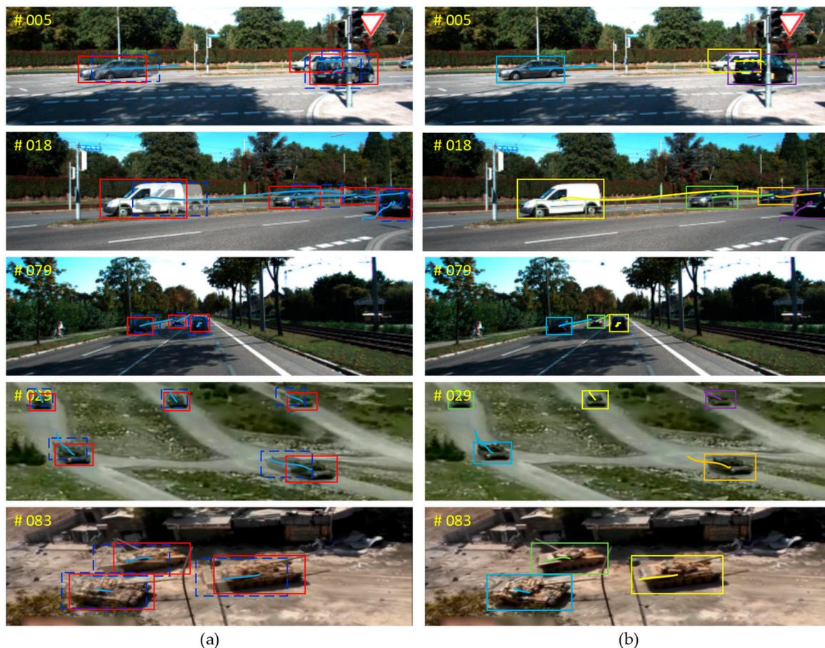
**Figure 10.** Experiment results using both the KITTI dataset and the ATTD. (a) Detection results with our Offline Candidates Recommendation Module. The previous position is denoted with a blue rectangle and the current with a red. (b) Tracking results using our MOT method and target trajectories.
