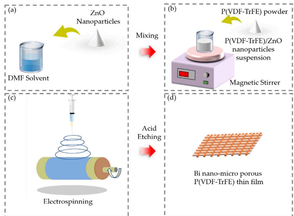
**Figure 1.** Schematic of the process for producing the pressure-responsive film by electrospinning and acid solution etching. (a) Mixing the ZnO nanoparticles; (b) dissolving the P(VDF-TrFE) powder. (c) Conceptual structure of electrospinning. (d) Responsive film after acid etching.
