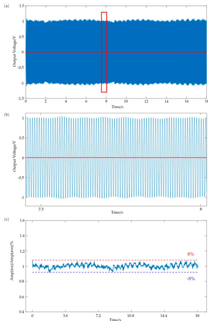
**Figure 7.** Schematic of the dynamic response of the flexible sensor. (a) Output voltage of the sensor versus time under a constant applied dynamic stimulus for 2500 cycles (frequency-140 Hz; SPL-95 dB). (b) Enlarged view of the output voltage waveform around 7.5–8 s. (c) The drift in Amp (ins) relative to Amp (ave).
