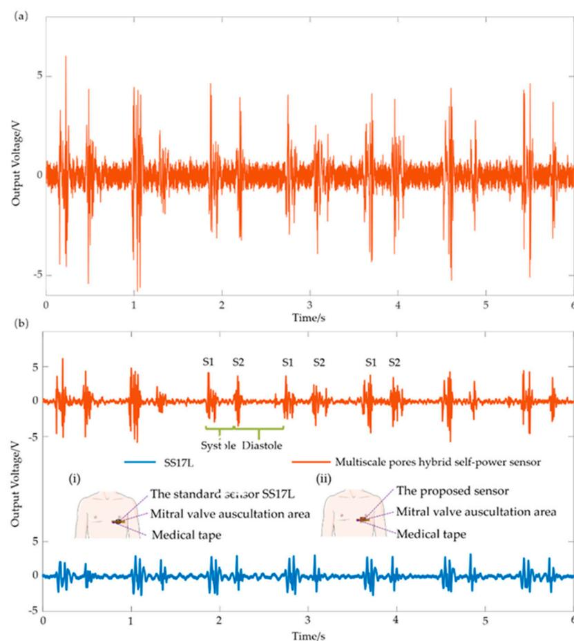
**Figure 10.** Schematic of heart sound detection in the human body. (a) Original signal of the heart sound signal; (b) heart sound signals after treatment with a filter. (i) Schematic drawing of the attachment of the standard sensor SS17L (BIOPAC, Goleta, CA, USA); (ii) schematic drawing of the attachment of the proposed flexible sensor.
