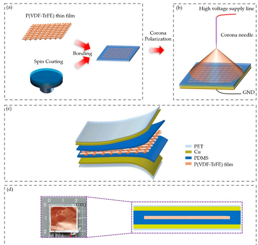
**Figure 2.** Schematic procedure for fabricating the flexible sensor. (a) PDMS sealing as the protective layers and electret layers. (b) Corona polarization. (c) Diagram of the sensor. (d) A sample measuring  $2 \times 2 \text{ cm}^2$  (left) and a cross-sectional diagram of the sensor's structure (right).
