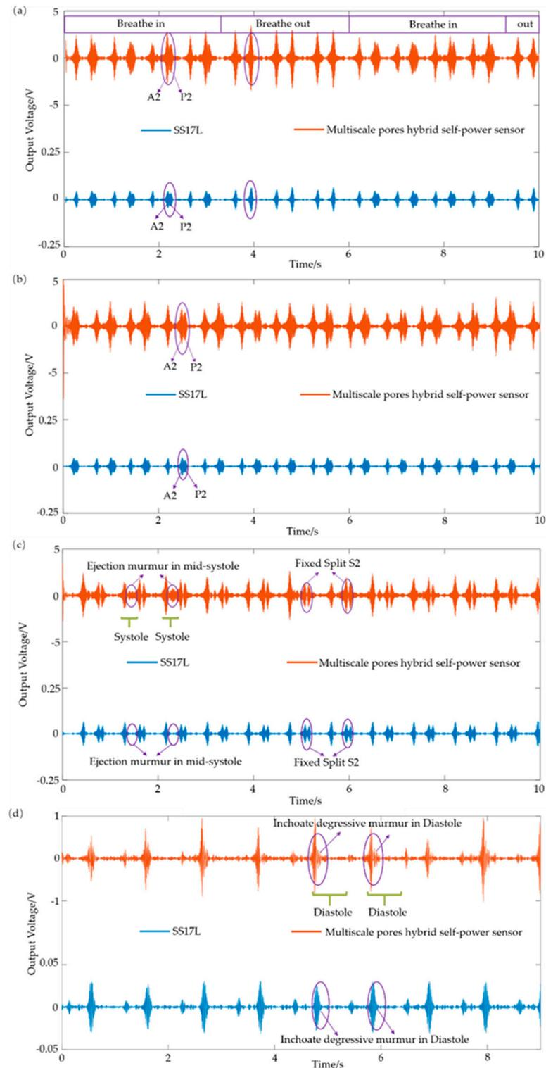
**Figure 9.** Schematic of pathological heart sound detection of SS17L (BIOPAC, Goleta, California, USA) and the proposed sensor. Representative features of (a) heart sound signal with a transient S2 split, (b) heart sound signal with a fixed S2 split, (c) heart sound signal of aortic regurgitation, and (d) heart sound signal of an atrial septal defect.
