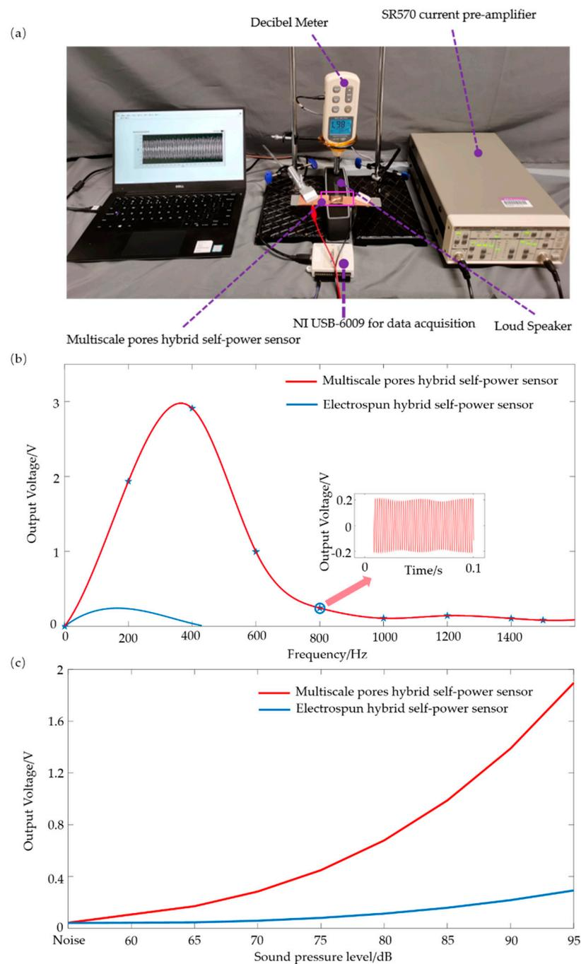
**Figure 6.** Schematic of the dynamic response of the flexible sensor. (a) Testing the dynamic stimulus system. (b) Responses of the sensors under changeable sound frequency (SPL-95 dB). (c) Responses of the sensors under a changeable SPL (frequency-200 Hz).
