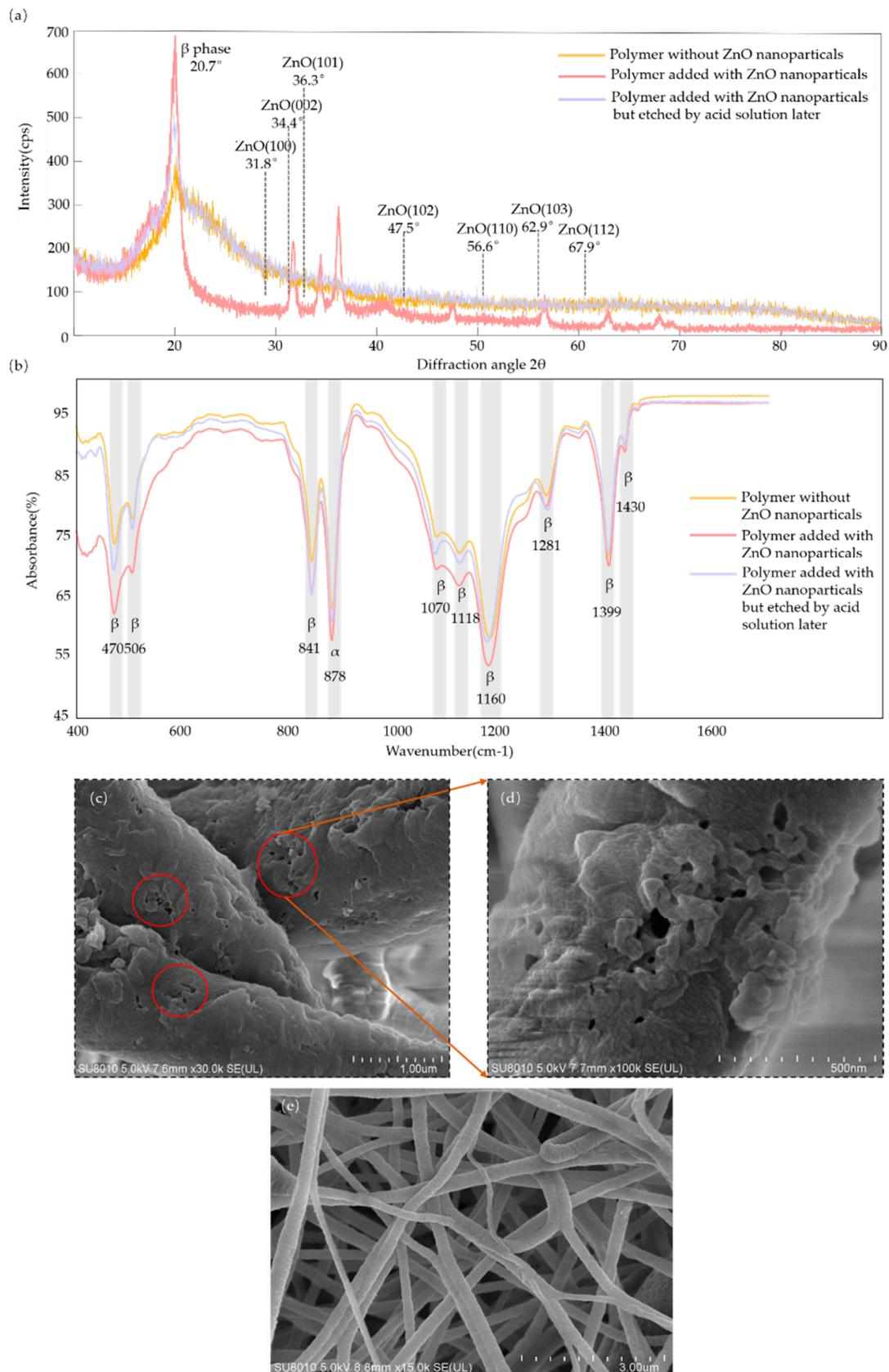
**Figure 3.** Schematic of analysis of the characteristics: (a) XRD spectra; (b) FTIR spectra of three kinds of P(VDF-TrFE) polymer film; (c) SEM image of nanoscale pores in the fibers (measuring scale in 1 micron). (d) Enlarged view of the nanoscale pores (measuring scale in 500 nm). (e) Overall morphology of the electrospinning fibers (measuring scale in 3 microns).
