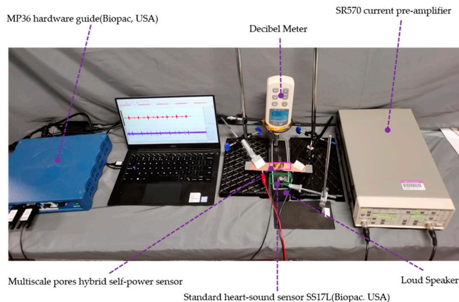
**Figure 8.** Schematic of the device for comparing the multiscale pore hybrid self-powered sensor and the standard heart sound sensor (SS17L, Biopac, Goleta, CA, USA).
