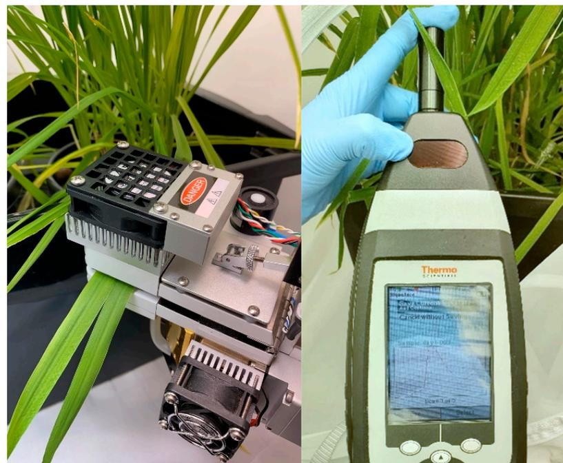
**Figure 2.** Photosynthetic gas exchange (**left**) and near-infrared (**right**) devices while taking measurements.
