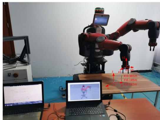
Figure 21. End effector displacements of Baxter's right arm on the real system.
