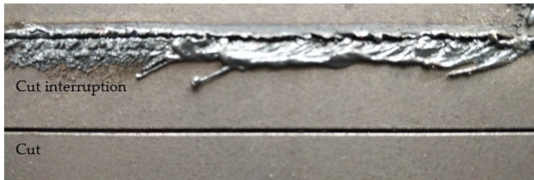
Figure 2. Top view of a metal sheet with a cut interruption ( top ) and complete cut ( bottom ).
