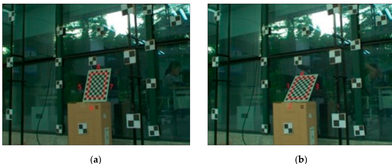
Figure 12. The image captured by camera 1. The eight 3D lines to be reconstructed are marked by the red lines on the images; (a) is more perpendicular and in a better intersection condition than (b).
