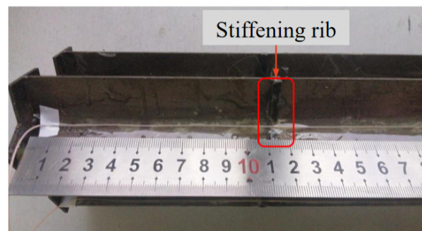
Figure 13. The fiber is jacked up at the stiffener rib.
