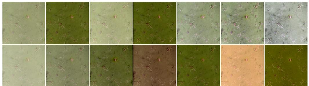
**Figure 3.** Example result of underwater image enhancement (left to right, starting from the top row): original raw image, DCP, MIP, RoWS, Paralenz, CLAHE, Fusion, GC, ICM, RGHS, UCM, UDCP, ULAP, TIP2016.
