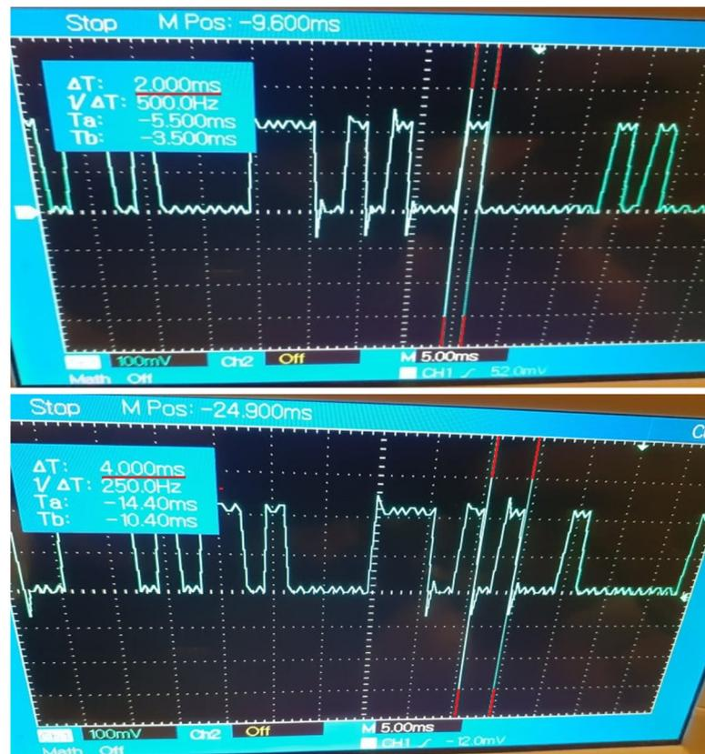
Figure 8. Generated Digital Signal based on payload delivered by the Gateway Application at 2 ms recurrence.
