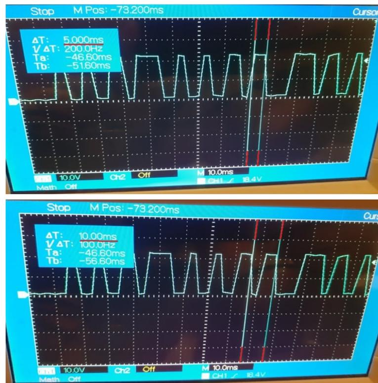
Figure 7. Generated Digital Signal based on payload delivered by the Gateway Application at 5 ms recurrence.
