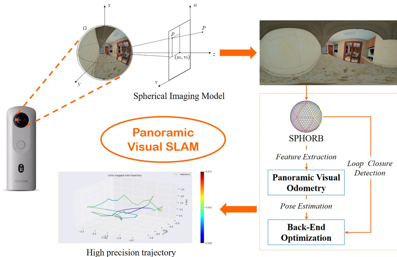
Figure 1. Flow chart of panoramic visual Simultaneous Localization and Mapping (SLAM).
