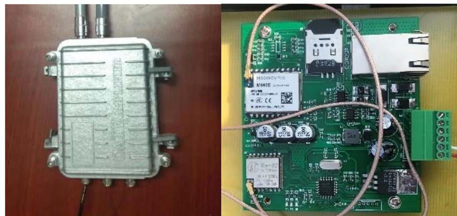
**Figure 7.** LoRa gateway installed on the construction site.
