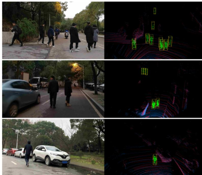
Figure 12. Typical experimental results on real road scenarios.
