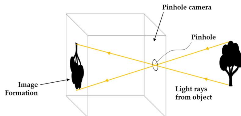
**Figure 6.** A graphical representation of the pinhole camera. The pinhole (aperture) restrains the light rays from the target from entering the pinhole; hence, affecting the brightness of the captured image (during image formation). A large pinhole (a wide opening) will result in a brighter image but is less clear due to blurriness on both background and foreground. Figure redrawn based on depictions in [132,133].
