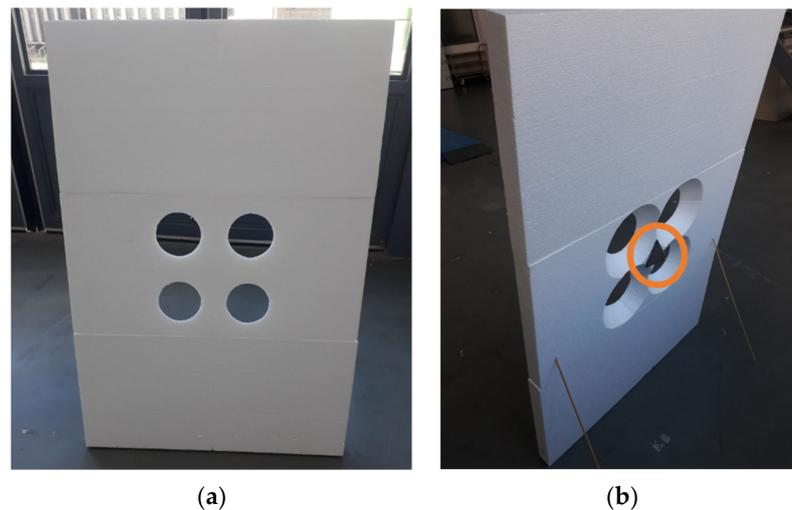
**Figure 9.** The proposed calibration target design to jointly extrinsic calibrate multiple sensors (radar, camera, LiDAR). It consists of four circular, tapered holes centrally located within a large rectangular board at the (a) front of the board, and a metallic trihedral corner reflector (circled in orange) located between the four circles at the (b) rear of the board. Figure source from [146,147] and modified.
