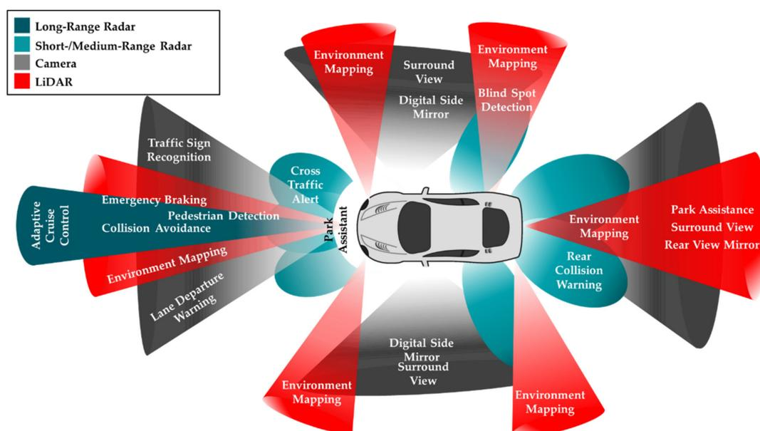
**Figure 3.** An example of the type and positioning of sensors in an automated vehicle to enable the vehicles perception of its surrounding. Red areas indicate the LiDAR coverage, grey areas show the camera coverage around the vehicle, blue areas display the coverage of short-range and medium-range radars, and green areas indicate the coverage of long-range radar, along with the applications the sensors enable—as depicted in [32] (redrawn).
