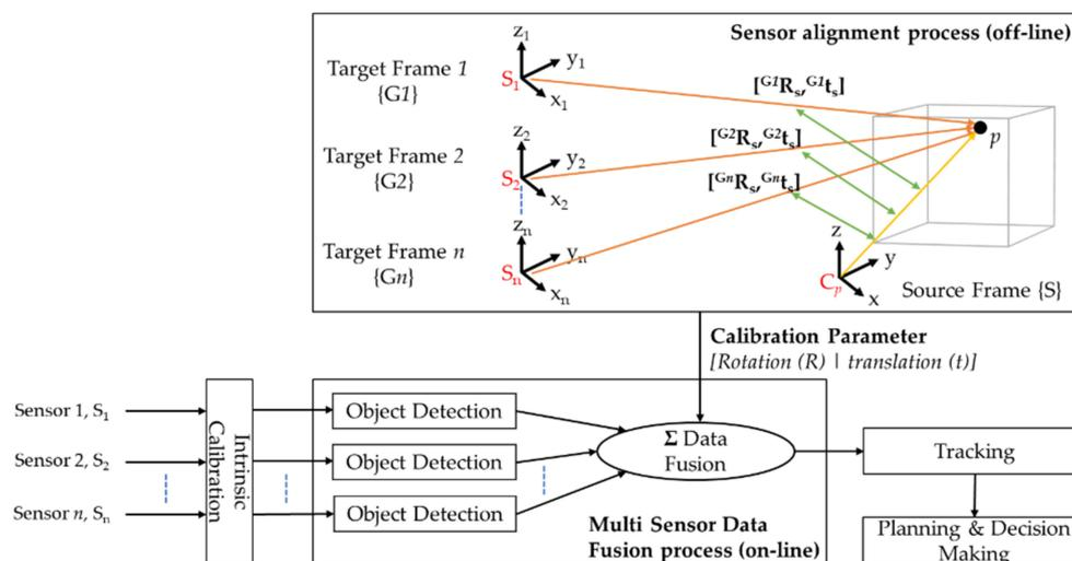
**Figure 5.** The structure of Multi-Sensor Data Fusion (MSDF) framework for  $n$  given sensors. It consists of a sensor alignment process (estimation of calibration parameters—rotation matrix and translations vector) and an object detection process which contains  $n$  processing chains, each provides a list of the detected obstacles. Figure redrawn based on depictions in [118], but with the inclusion of an intrinsic calibration process.
