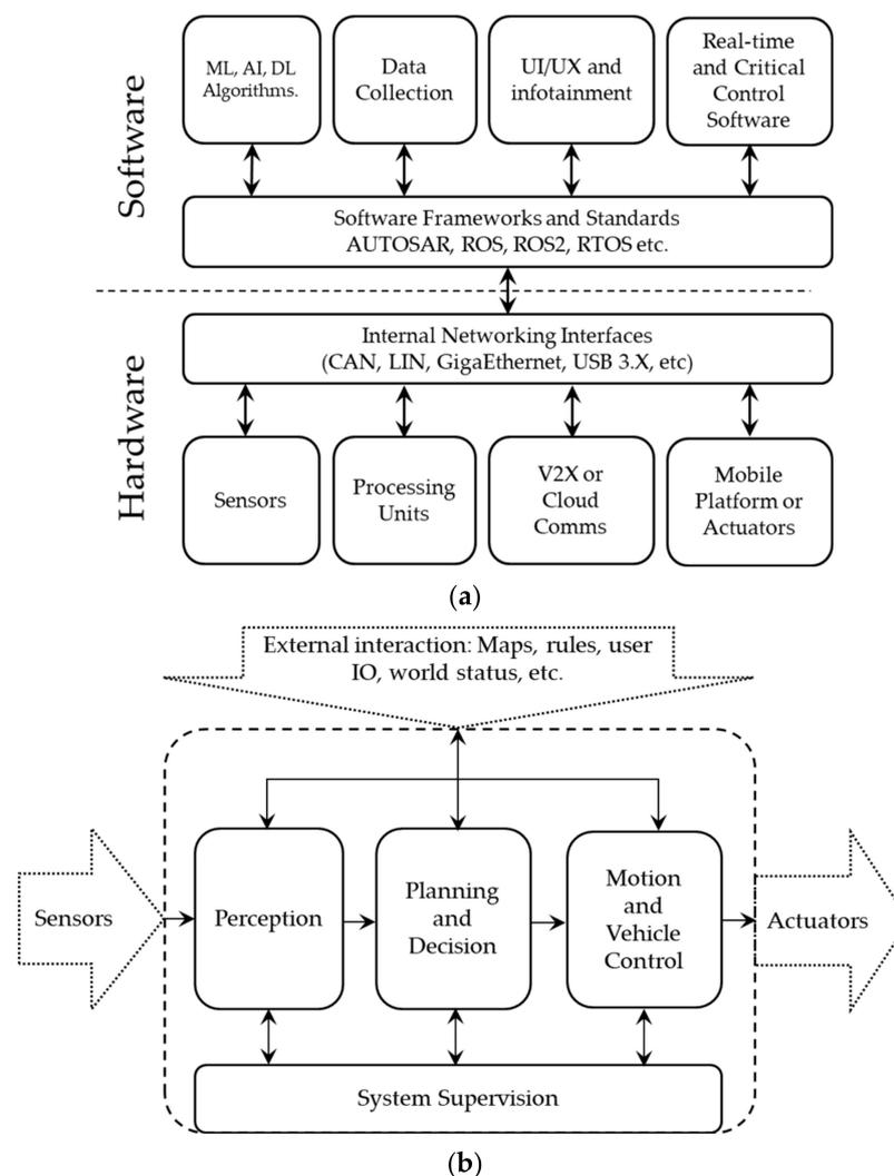
**Figure 2.** Architecture of an autonomous driving (AD) system from, (a) a technical perspective that describes the primary hardware and software components and their implementations; (b) a functional perspective that describes the four main functional blocks and the flow of information based on [15].
