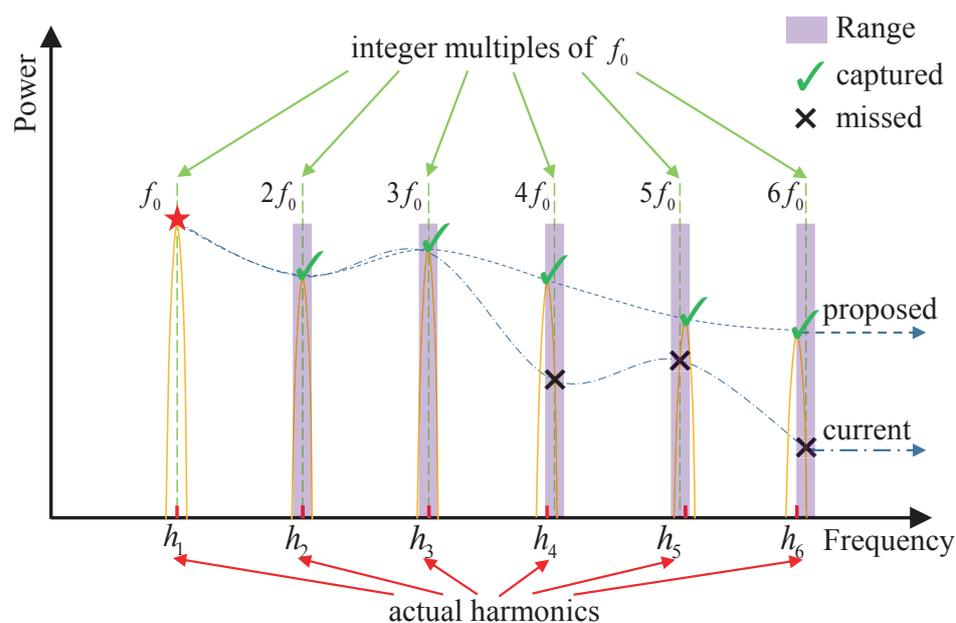
**Figure 4.** Modeling harmonic structure with loose constraint.
