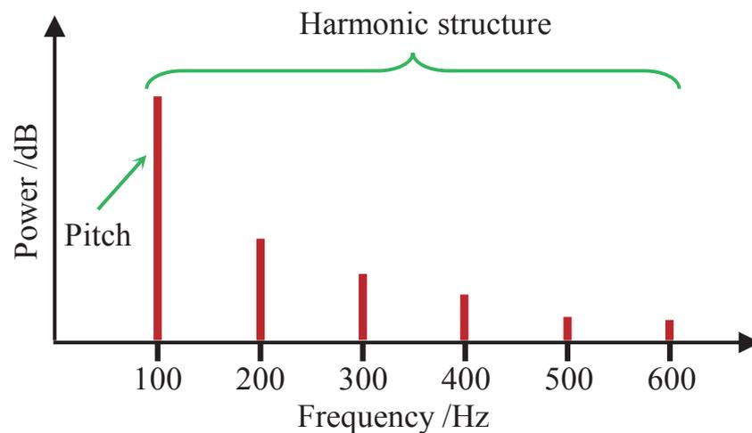
**Figure 1.** Harmonic structure of audio signal.
