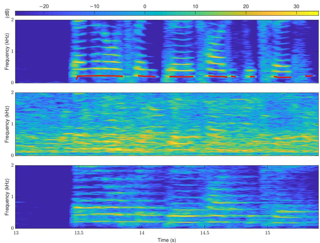
**Figure 2.** Smooth prior of pitch trajectory. The spectrogram corresponds to a segment of speech signal named “f1nw0000.pes” in the Keele database. The upper one is clean speech, wherein the red lines are pitch trajectories. The middle one is under babble noise of  $-5$  dB SNR. The lower one is under  $RT60 = 1.0$  s, and the other conditions are the same as the subsequent experiment.
