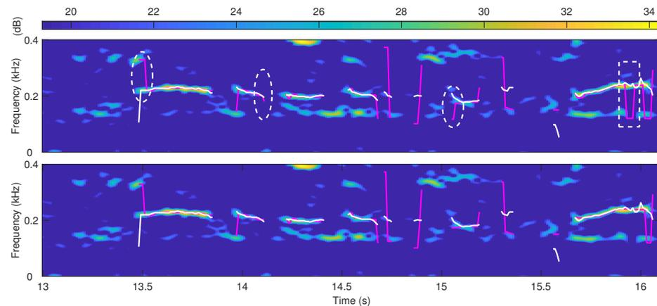
**Figure 6.** Pitch estimation of the proposed method without the segment extension approach (the upper) and with the segment extension approach (the lower). The spectrogram and the ground truth correspond to a segment of speech signal named “f1nw0000.pes” in the Keele database. The white lines are ground truths, and the red lines are the estimated results. The speech is mixed with babble noise of  $-5$  dB SNR.
