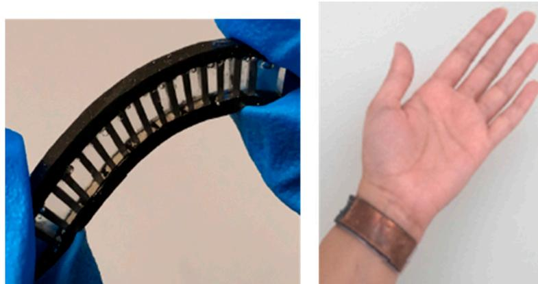
**Figure 4.** Thermoelectric device with n- and p-type off-the-shelf thermoelectric legs sprayed eutectic gallium indium (EGain) liquid metal for interconnects and encased in PDMS (**left**). Device coated with copper to distribute heat (**right**) [49]. Reproduced with permission from Appl. Energy. Copyright 2020 Elsevier.
