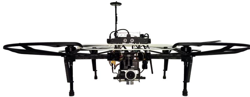
**Figure 5.** The robot developed for our project. The figure shows our DJI Matrice 100 quadrotor equipped with the indoor testing parts (DJI Guidance System and the propeller guards), as well as the DJI Zenmuse X3 Gimbal and Camera system, the SF30 altimeter, and the DJI Manifold onboard computer.
