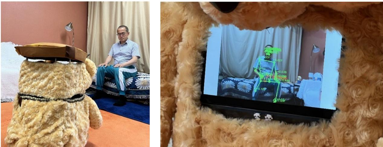
**Figure 10.** Left: Dori and the user under monitoring service. Right: Skeletal model is extracted from camera image using MediaPipe Pose.
