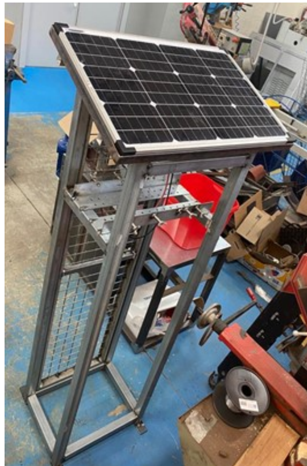
Figure 8. Storage structure for the air quality monitoring sensors in its development stage.
