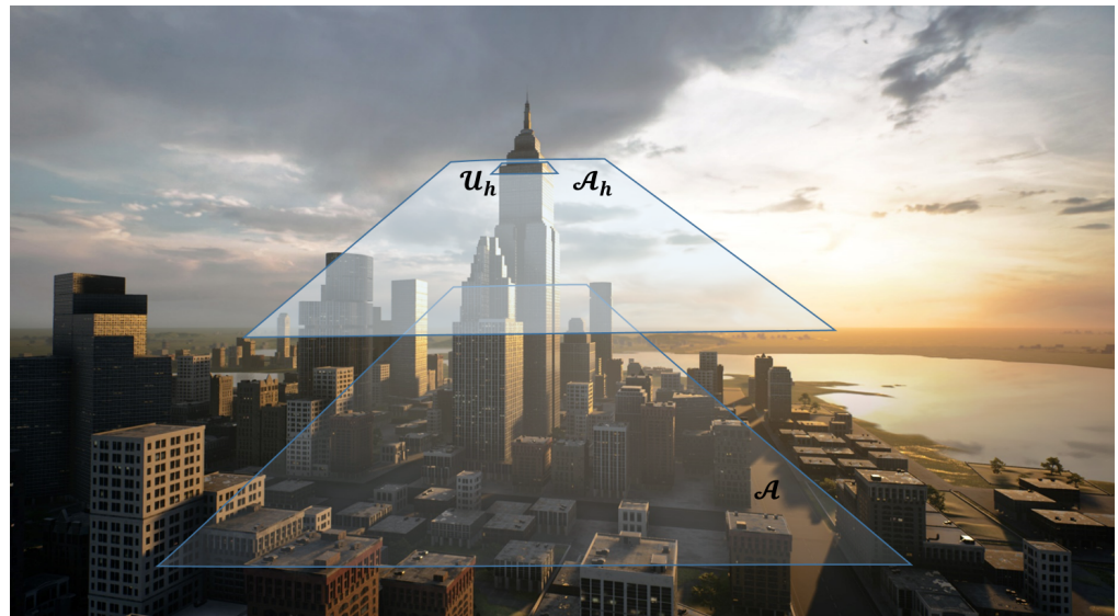
Figure 2. The area of interest \mathcal{A} , the plane \mathcal{A}_h at an altitude h , and the mapping of an obstacle \mathcal{U}_h .
