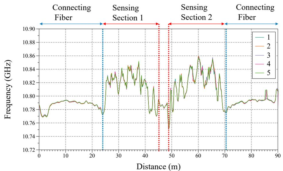
**Figure 6.** Baseline frequency response on Grist Mill Bridge without loading.
