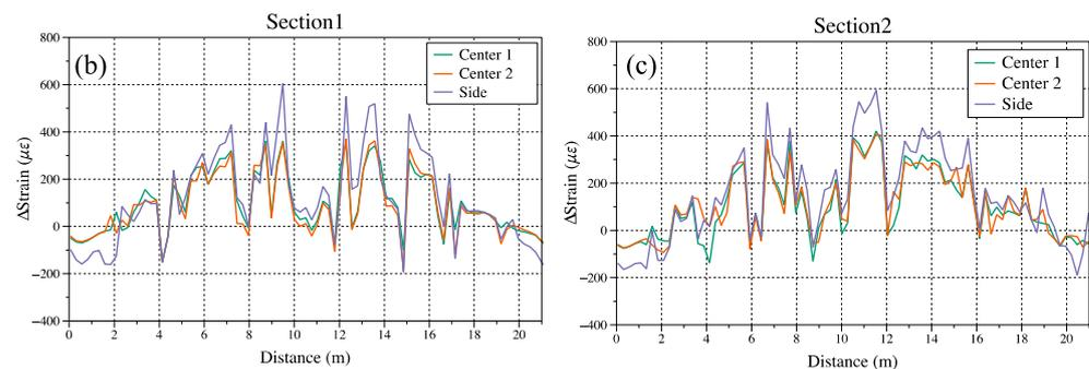
**Figure 9.** Comparison of different loading test results on sensing Sections 1 and 2. (a) Strain distribution results of Baseline and loading tests. (b) Strain difference between loading tests and baseline in Section 1. (c) Strain difference between loading tests and baseline in Section 2.
