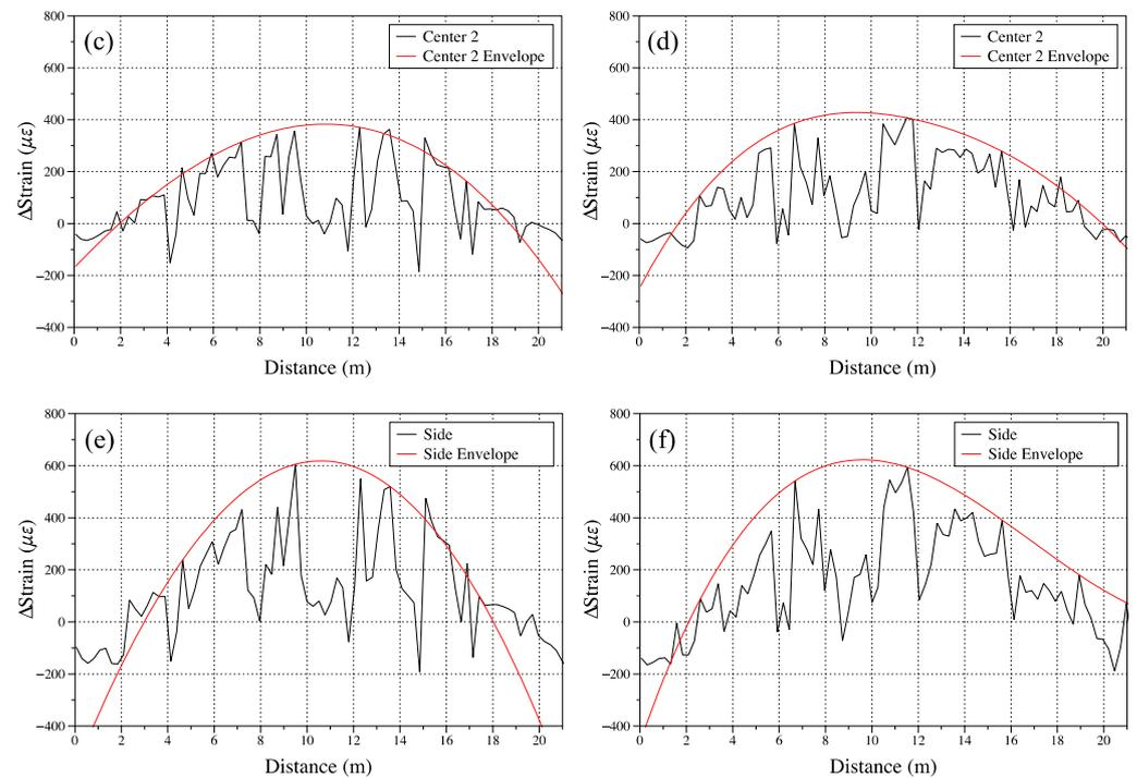
**Figure 8.** Strain distribution of different loading tests. (a,b) Experiment results of sensing Sections 1 and 2 on the first loading test with the trucks located in the center of the bridge. (c,d) Experiment results of the sensing Sections 1 and 2 on the second loading test with the trucks located in the center of the bridge. (e,f) Experiment results of sensing Sections 1 and 2 on the loading test with the trucks located on one side of the bridge.
