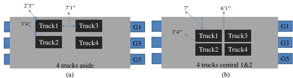
**Figure 7.** Schemes of the loading tests. (a) The first test of four trucks located close to one side of the bridge. (b) Second and third tests of four trucks located in the center of the bridge.
