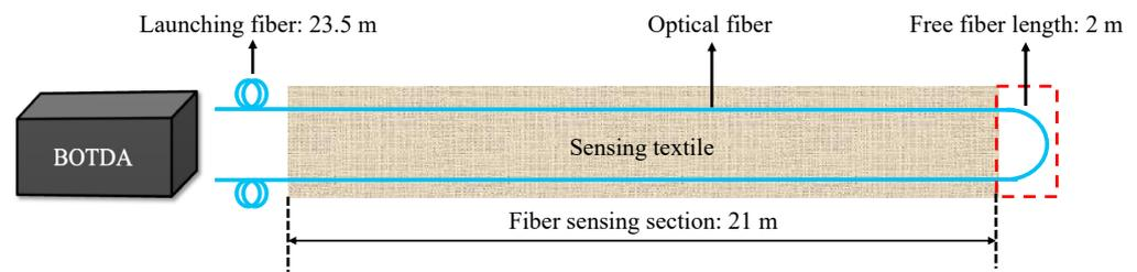
**Figure 1.** Schematic of the fiber optic sensing textile design.
